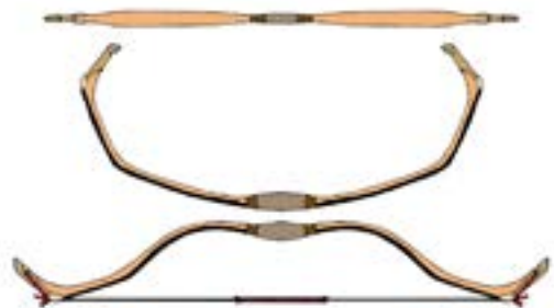
Figure 9. The Kazakh lesser horsebow (of Crimean-Tartar type). Reconstruction by author
